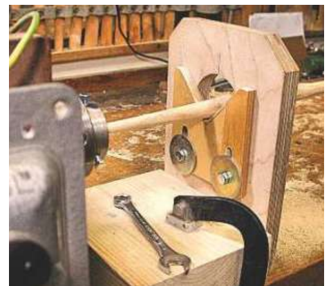
▲ Pic. 4 The adjustable support is useful when working slender stuff
